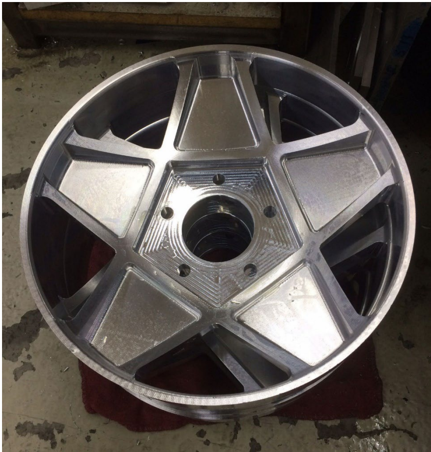
Recreation wheel center section being CNC Machined – Race Concepts.
