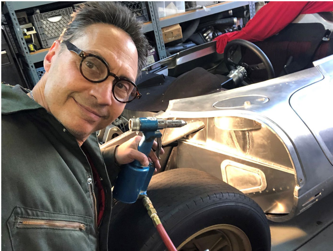
John Nino installing the 1800+ rivets.
