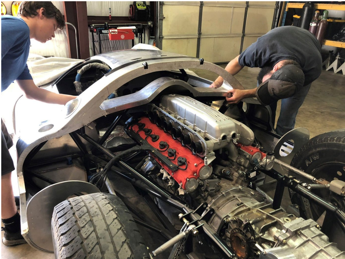
Wesley Taylor and Joe Maher – Reassembling the body with the fresh F550 V12 Installed – Red Car Restorations.
