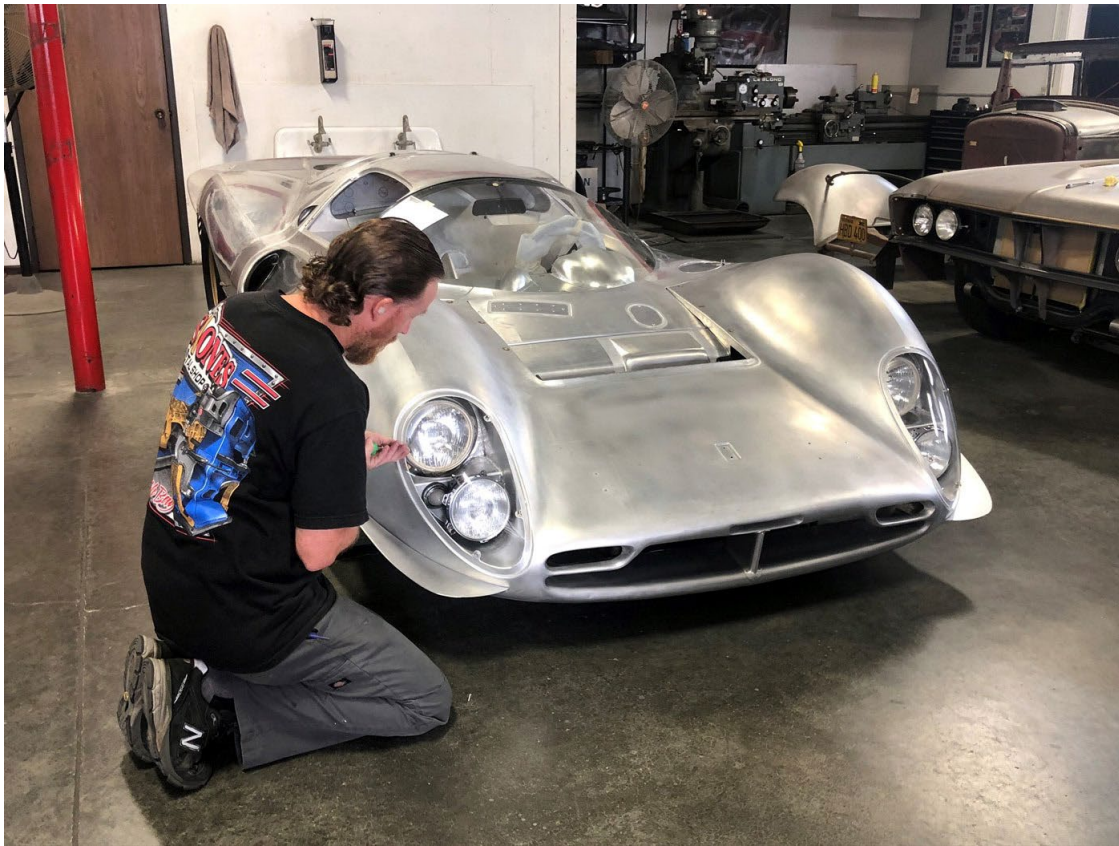
Brian Stone – Stone's Metal Shop – Installation of P4 Headlight Perspex from David Piper's Collection.
