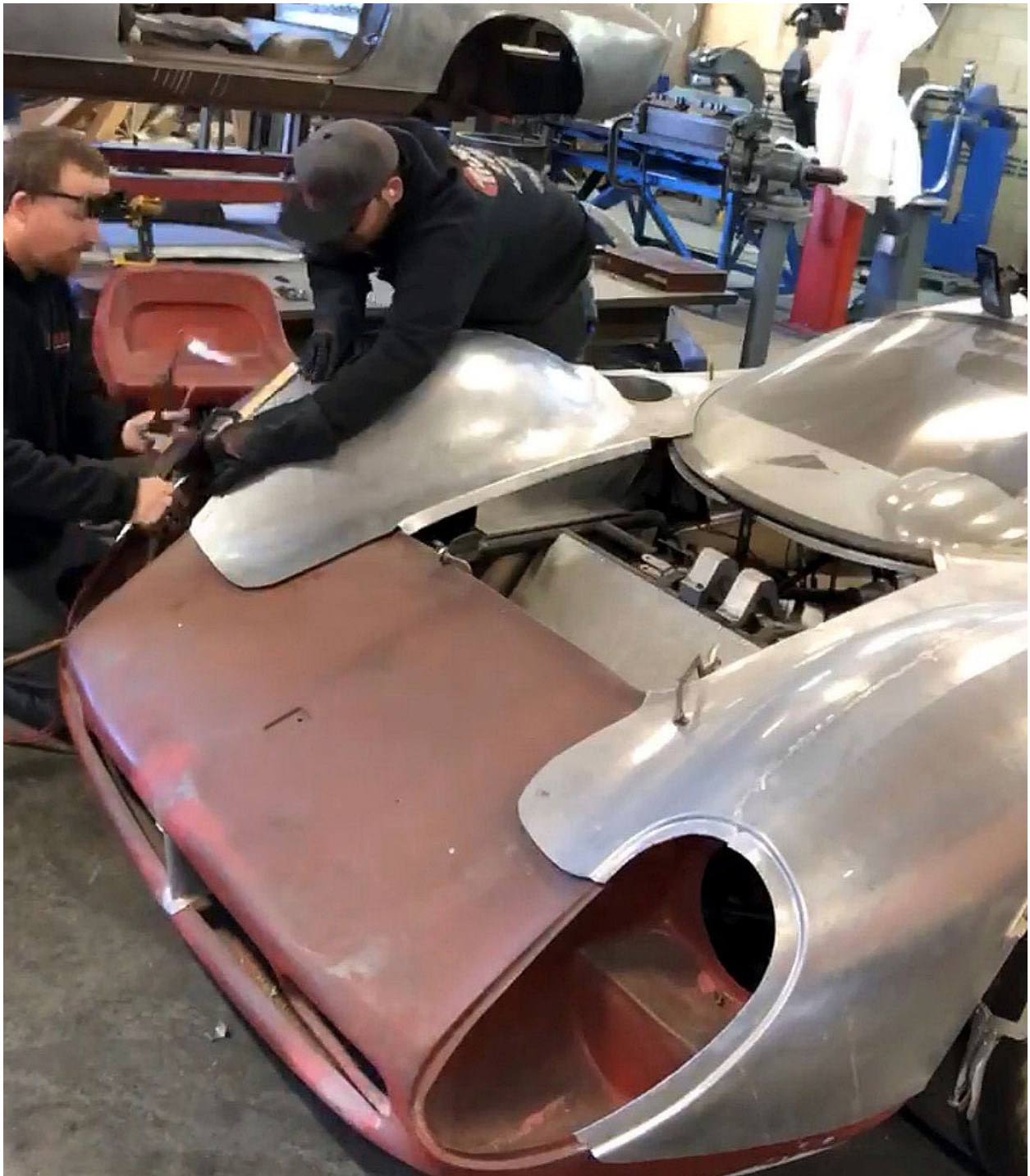
Brian Stone and Geoff Monise – Stone’s Metal Shop, accurately recreating 412P nose section in aluminum.
