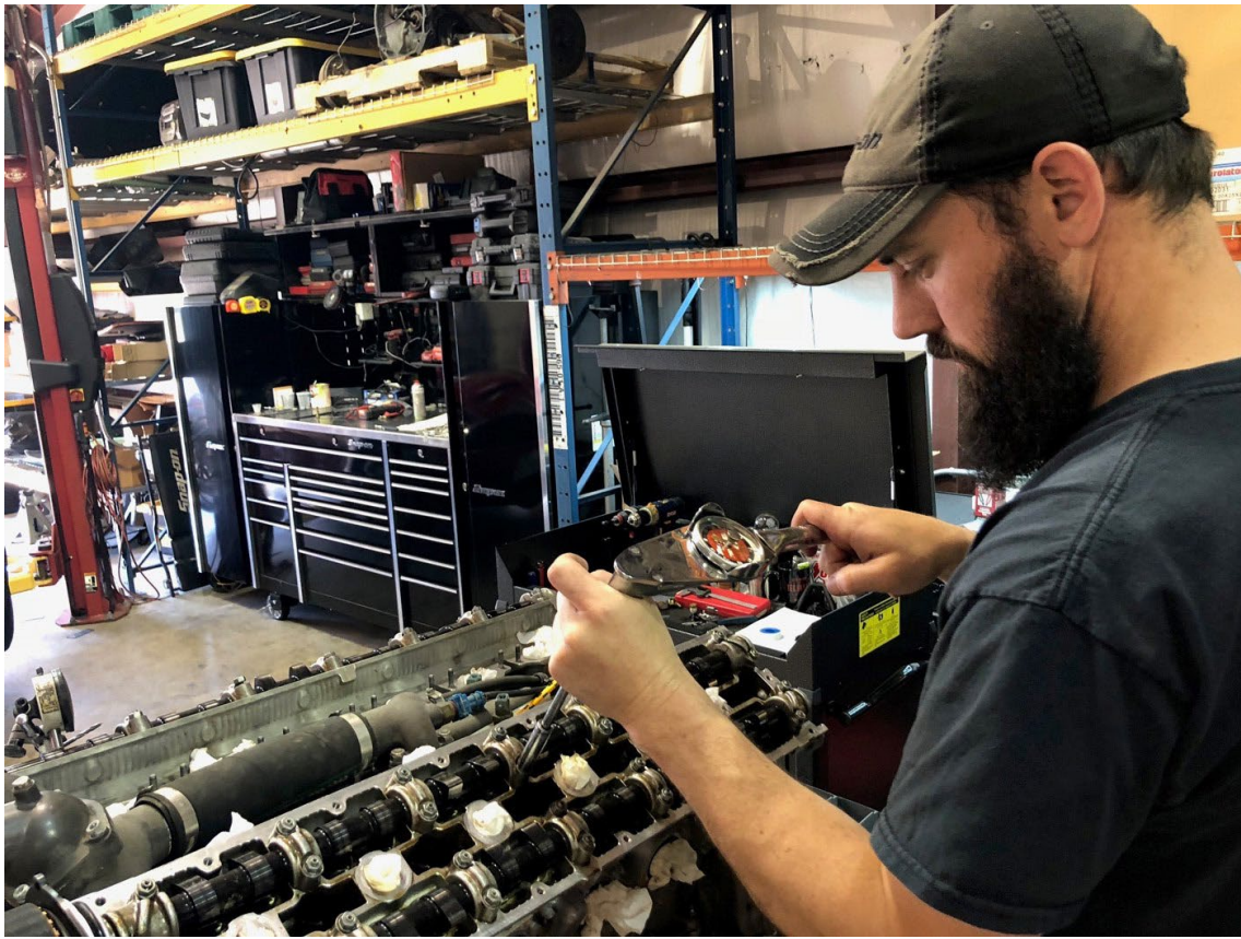
Joe Maher – Reassembling the Ferrari F550 V12 Engine – Red Car Restorations.
